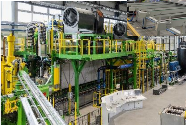
New press with a pressure of 4000T in Kęty (EPS)
